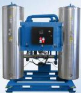
The Heat Of Compression air dryers represent the more efficient compressed air drying technology available today. They recover the heat produced by the process of compression that, instead of being dissipated in the environment, is used in the drying process to provide dry air without consuming energy or compressed air. In fact, the only operating cost is the power required for the control system.
